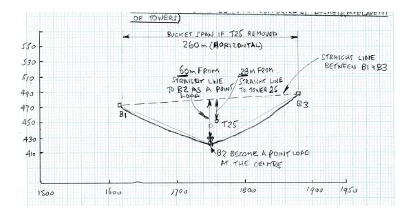
Spacing of buckets (See 1.1) Thus, Haul rope span, no centre bucket Horizontal span (See Sketch 2) Rope tension T2 at the creek (See 2.3.2) Empty bucket weight (See 1.1) Sag (from "HaulRopeCatenary.xlxs") 140 m 280 m 260 m 3.88 kN 2.04 kN 60 m (see Sketch 2)
